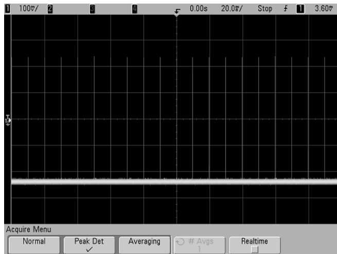
15 ns Narrow Pulse, 20 ns/div, Peak Detect Mode
